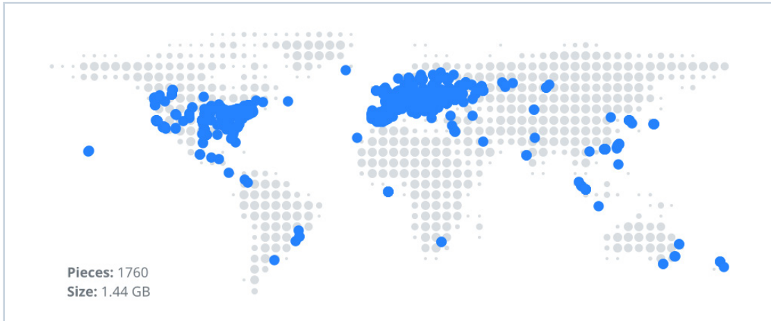
Figure 2: Storj Object Map. This image shows the approximate location of Storj points of presence storing 1,760 encrypted erasure-encoded pieces of a 1.44GB object. Only a subset of the nearest pieces are required to reconstitute the original object.
