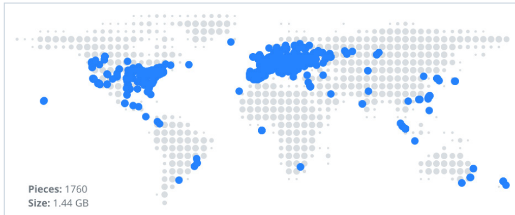
Figure 1: Storj Object Map. This image shows the approximate location of Storj points of presence storing 1,760 encrypted erasure-encoded pieces of a 1.44GB object. Only a subset of the nearest pieces are required to reconstitute the original object.
